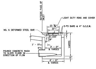
REINFORCING BARS USED IN THE INLET SHALL BE \*4 BARS @ 10" O.C. BOTH WAYS.
