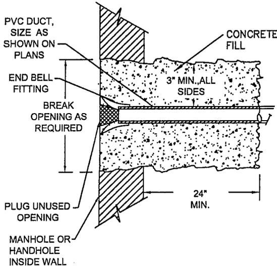
**DUCT ENTRY DETAIL AT MANHOLES AND HANDHOLES**
