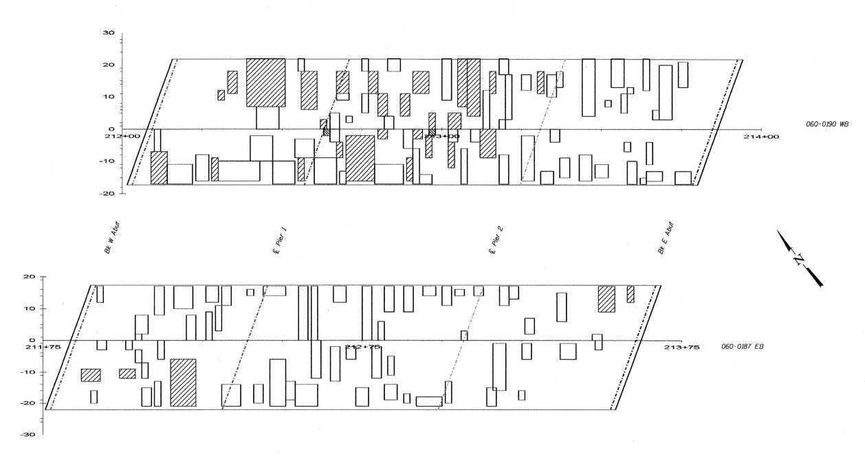
DECK SLAB REPAIR (FULL DEPTH, TYPE I) 0.9 SY
