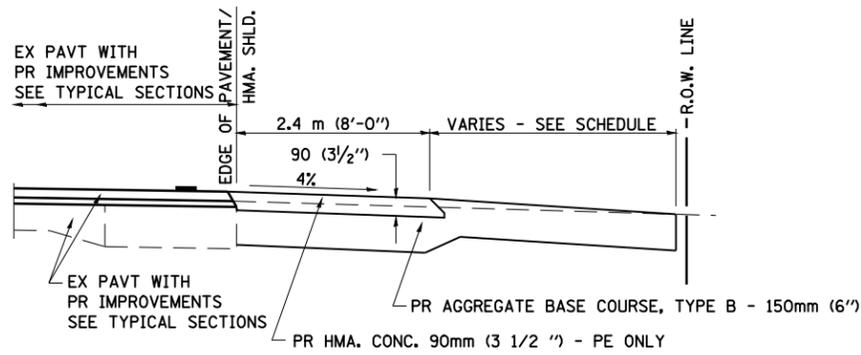
**SECTION A-A FOR EX EARTH/AGGREGATE FE & PE**
