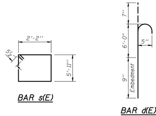
\* EPOXY GROUT BARS IN 9" MIN. HOLES ACCORDING TO ARTICLE 584 OF THE STANDARD SPECIFICATIONS.
