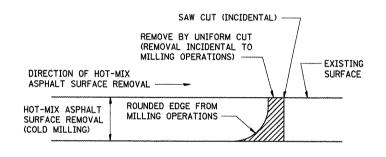
NOTE: WHEN MILLING OPERATIONS PRODUCE A ROUNDED EDGE,
