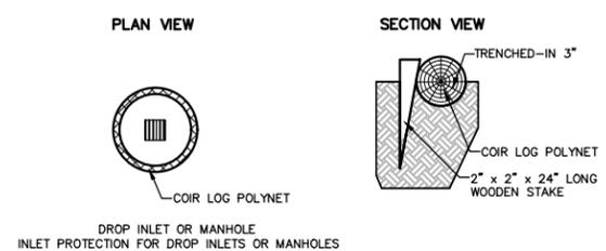
\* USE 9LB DENSITY 12" DIAMETER, 20' LONG COIR LOG POLYNET FOR STANDARD CIRCULAR DRAINAGE STRUCTURES. PLACE THE COIR LOG AROUND THE STRUCTURE AND JOIN THE ENDS TOGETHER WITH COIR TWINE. USE 2"x2"x24" WOODEN STAKES SPACED 3' APART TO HOLD DOWN LOG POLYNET.
