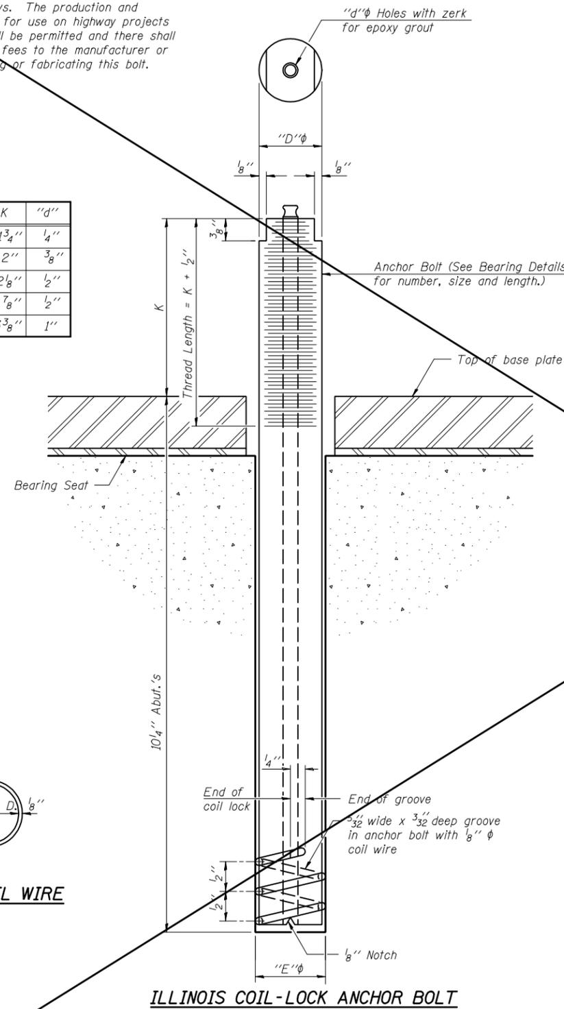
**MATERIALS FOR ILLINOIS COIL-LOCK ANCHOR BOLT**
