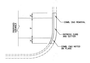
PROPOSED DEPRESSED CURB & GUTTER EXISTING CURB & GUTTER NOT DEPRESSED NOT TO SCALE
