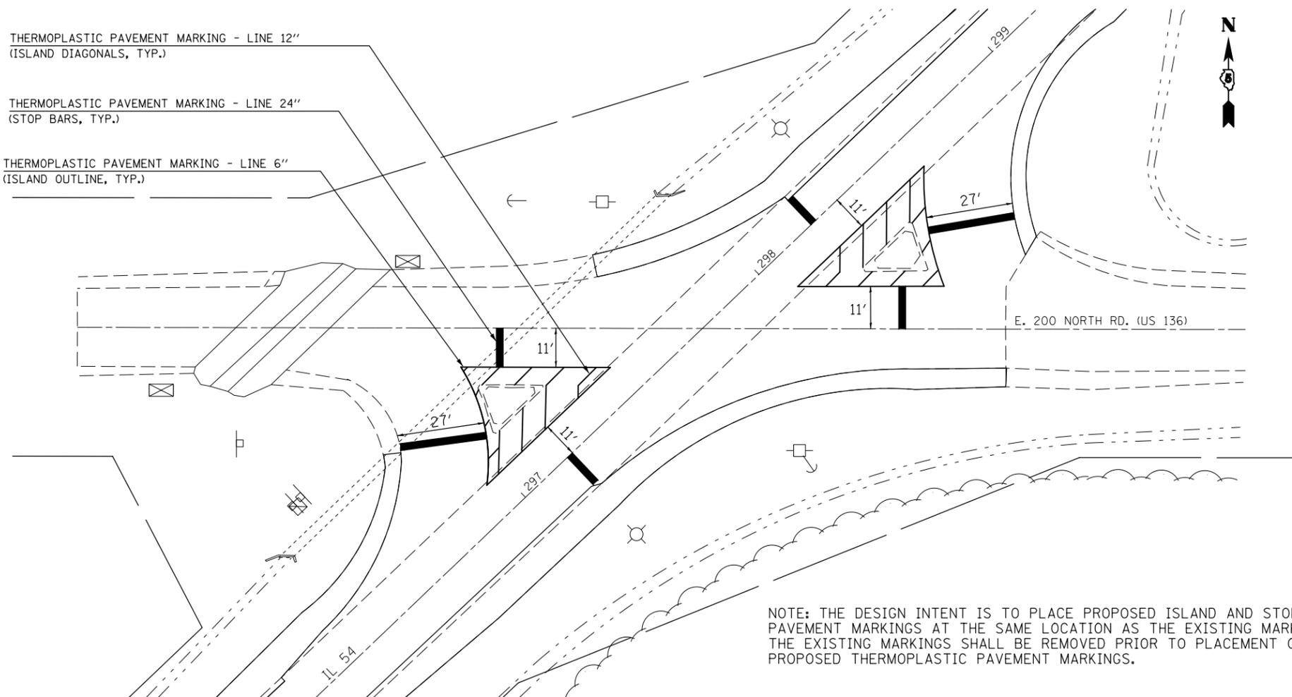
NOTE: THE DESIGN INTENT IS TO PLACE PROPOSED ISLAND AND STOP BAR PAVEMENT MARKINGS AT THE SAME LOCATION AS THE EXISTING MARKINGS. THE EXISTING MARKINGS SHALL BE REMOVED PRIOR TO PLACEMENT OF THESE PROPOSED THERMOPLASTIC PAVEMENT MARKINGS.
