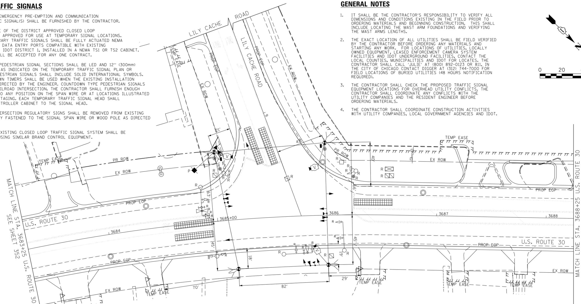
6. IF NO TRAFFIC STAGING IS IN PLACE OR WILL NOT BE STAGED ON THE DAY OF THE TURN ON, THE TEMPORARY TRAFFIC SIGNAL SHALL HAVE THE SIGNAL HEAD DISPLAYS, SIGNAL HEAD PLACEMENTS AND CONTROLLER PHASING MATCH THE EXISTING TRAFFIC SIGNAL AT THE TIME OF THE TURN-ON.
