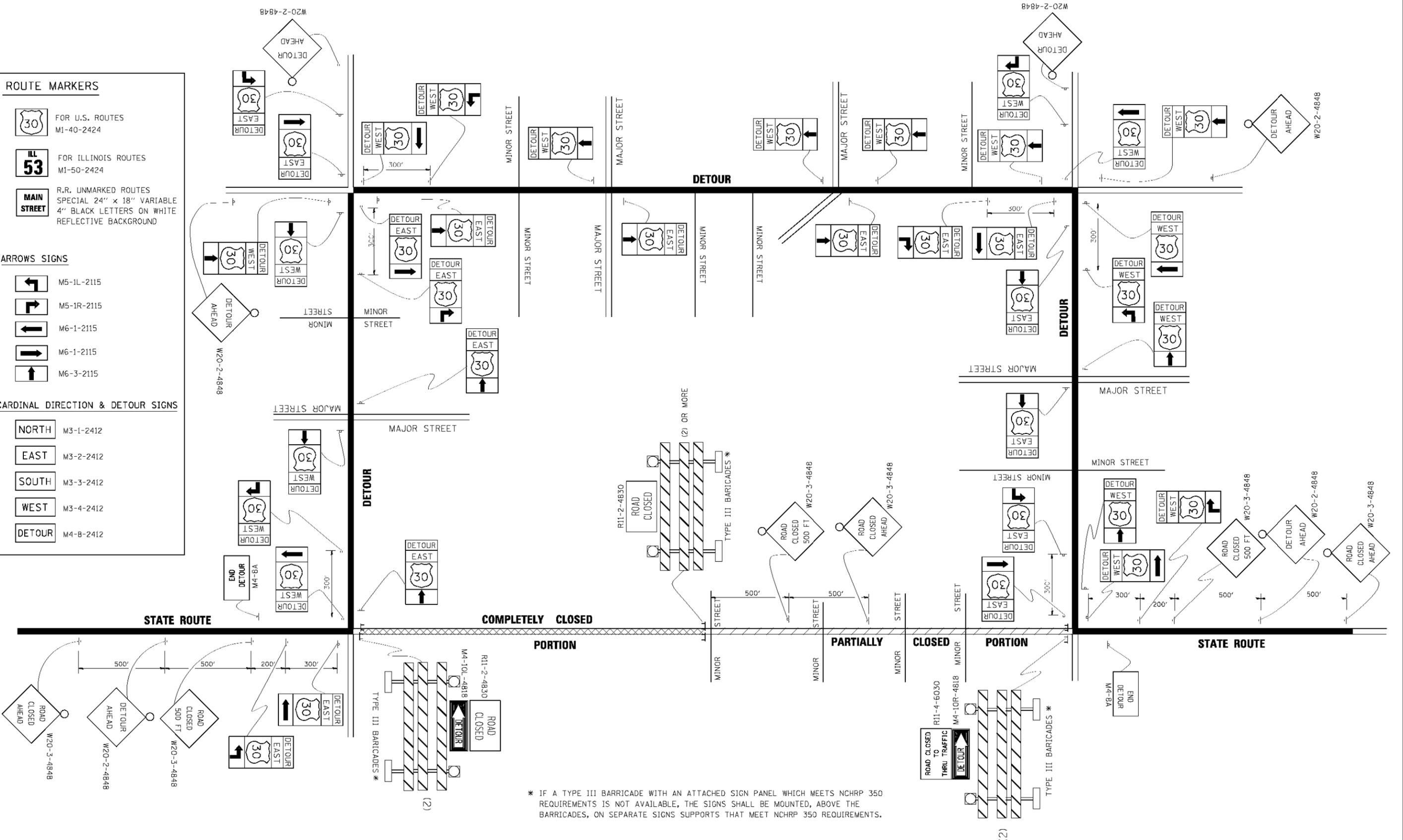
\* IF A TYPE III BARRICADE WITH AN ATTACHED SIGN PANEL WHICH MEETS NCHRP 350 REQUIREMENTS IS NOT AVAILABLE, THE SIGNS SHALL BE MOUNTED, ABOVE THE BARRICADES, ON SEPARATE SIGNS SUPPORTS THAT MEET NCHRP 350 REQUIREMENTS.
