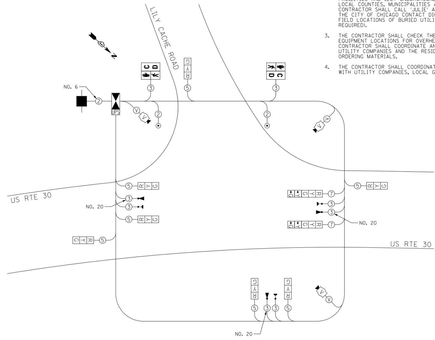
SIGNAL HEADS SHALL BE SHIFTED ALONG TEMPORARY SIGNAL SPAN WIRE AS APPLICABLE TO THE ASSOCIATED MOT STAGE.
