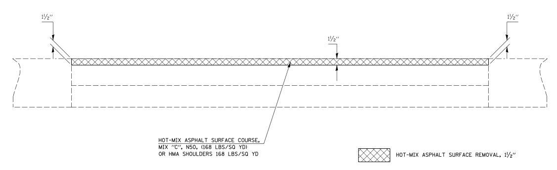
DESIGNED - BJH REVISED FILE NAME = USER NAME = hoganbj STATE OF ILLINOIS i50-sht-details.dgr DRAWN BJH 8/31/2010 REVISED MILLING AND PAVING TRANSITION DETAILS (57-20(1),21,22)RS-3 McLean 150 85 CHECKED REVISED **DEPARTMENT OF TRANSPORTATION** CONTRACT NO. 70550 SCALE: SHEET NO. 10 OF 10 SHEETS STA. PLOT DATE = 10/21/2010 DATE REVISED
