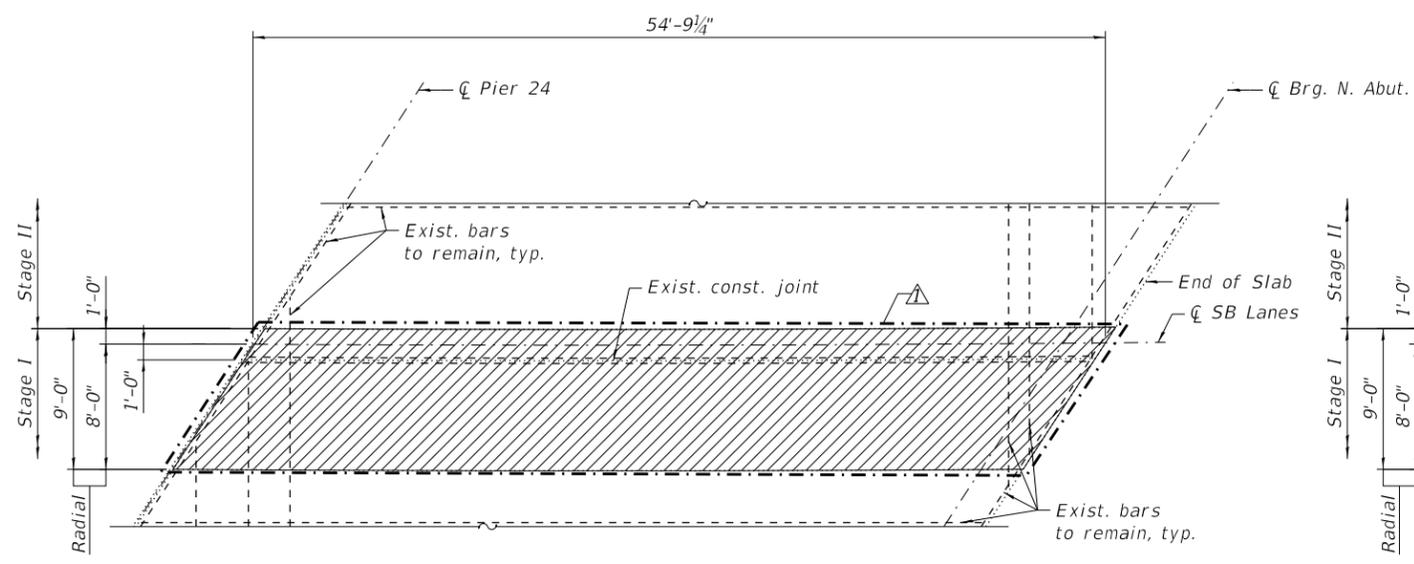
**PARTIAL DECK PLAN REMOVAL (SPAN 25)**
