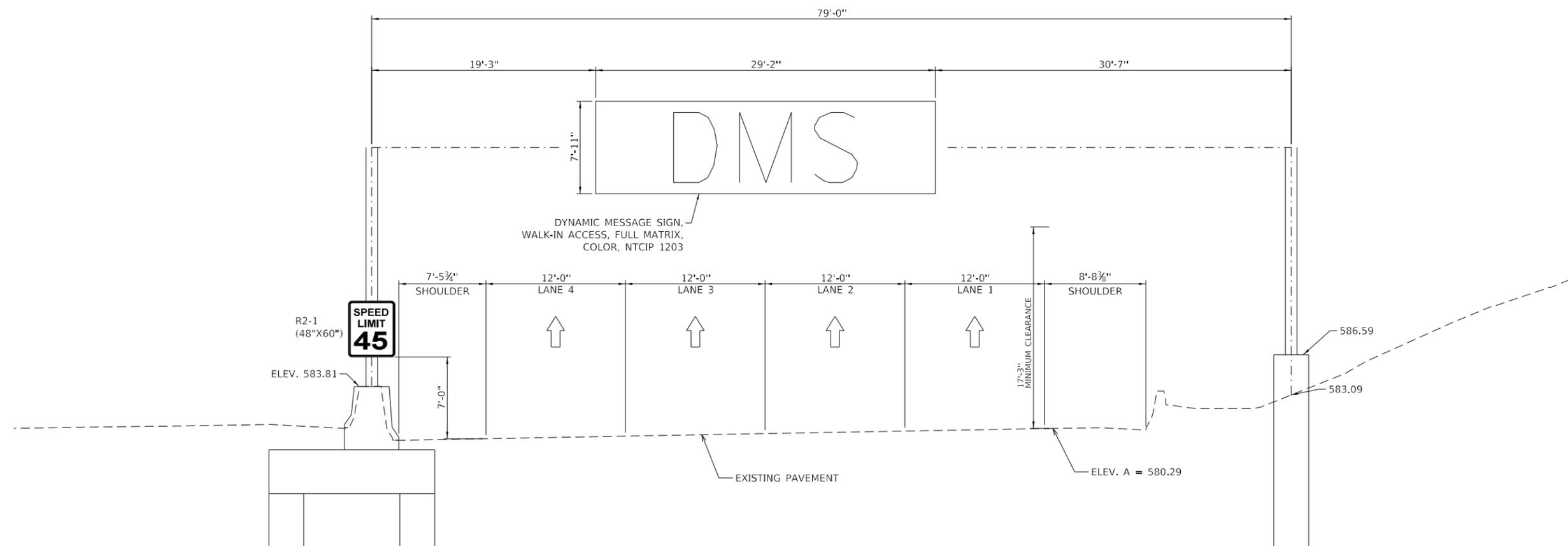
**SIGN 16 (CM13) STA 344+53.87 (SB) - PROPOSED SIGN TRUSS MOUNT**
