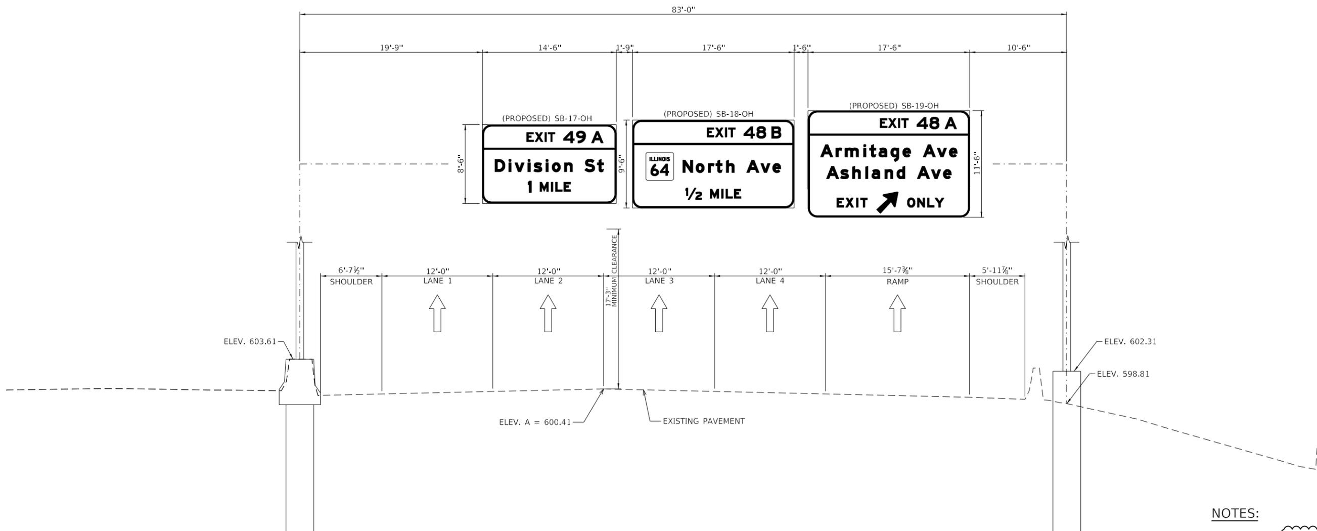
SIGN 9 STA 425+40.12 (SB) - PROPOSED SIGN TRUSS MOUNT
