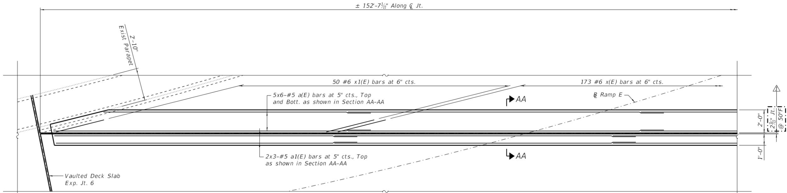
**WEST ABUTMENT JOINT RECONSTRUCTION PLAN**
