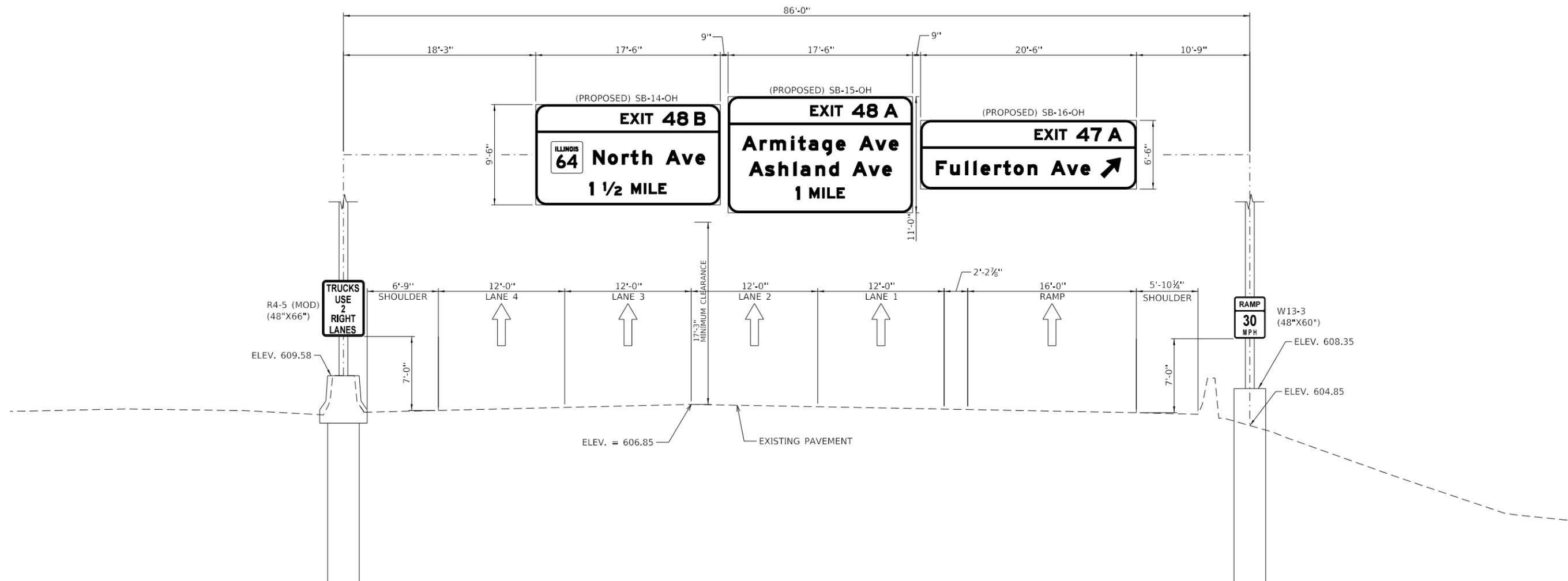
SIGN 8 STA 471+82.88 (SB) - PROPOSED SIGN TRUSS MOUNT
