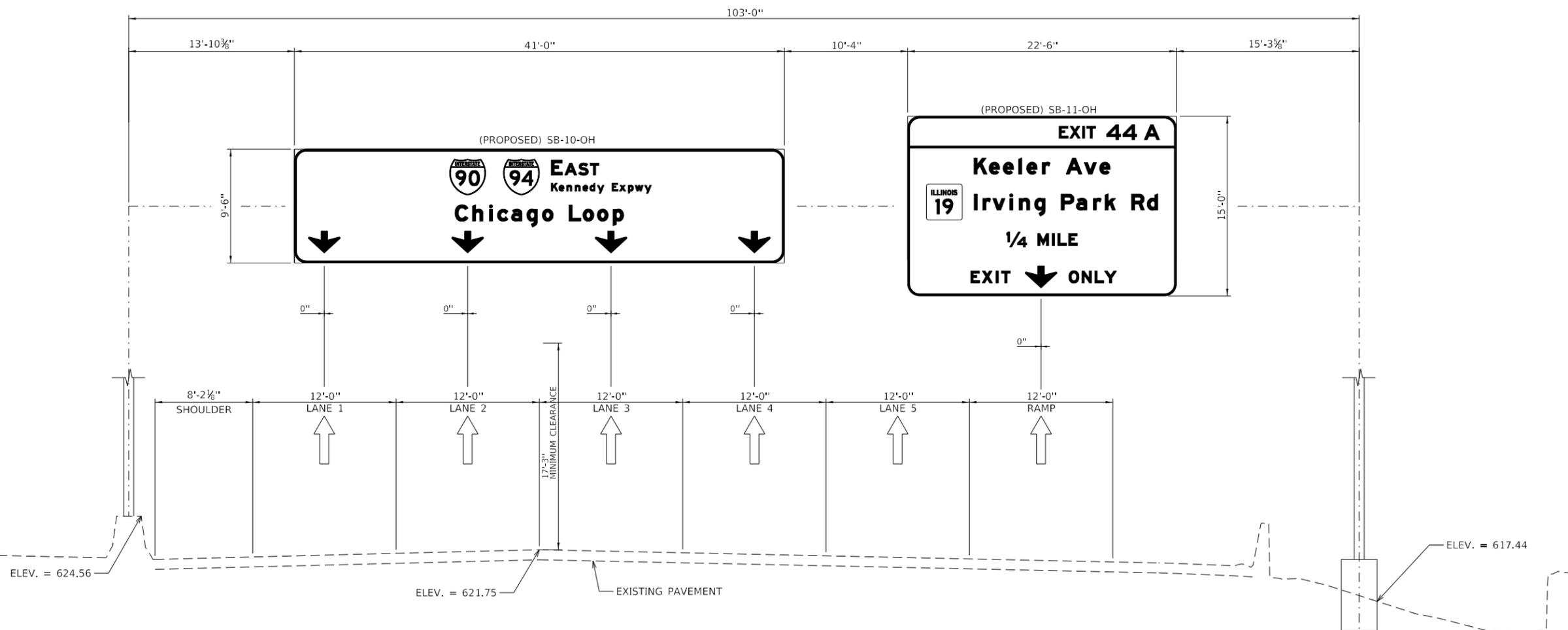
SIGN 6 STA 655+85.00 (SB) - PROPOSED SIGN TRUSS MOUNT
