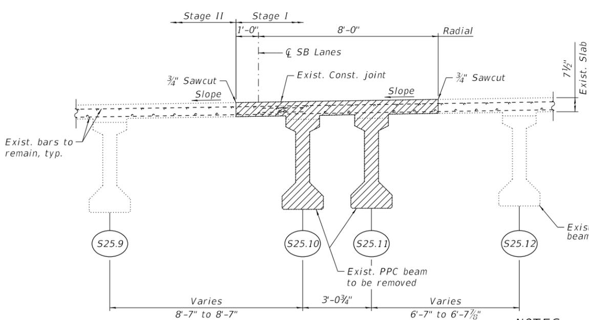
**PARTIAL CROSS SECTION REMOVAL (SPAN 25)**
