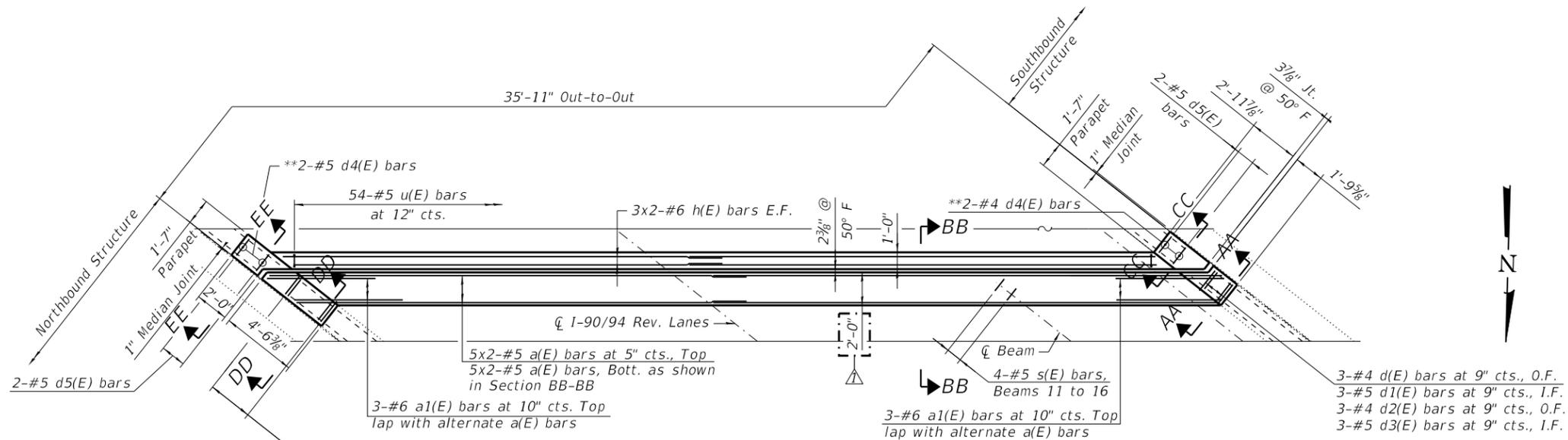
**SOUTH ABUTMENT JOINT RECONSTRUCTION PLAN**
