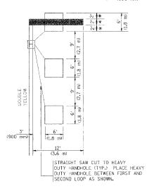
NOTE: DUAL LEFT TURNS NOT SHOWN REFER TO PLAN SHEET FOR DETECTOR LOOP REPLACEMENT
