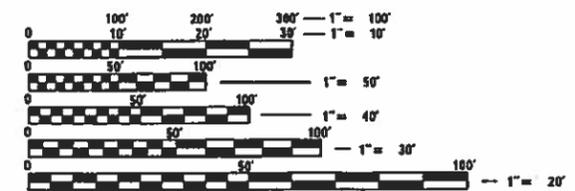
FULL SIZE PLANS HAVE BEEN PREPARED USING STANDARD ENGINEERING SCALES. REDUCED SIZED PLANS WILL NOT CONFORM TO STANDARD SCALES. IN MAKING MEASUREMENTS ON REDUCED PLANS, THE ABOVE SCALES MAY BE USED.
