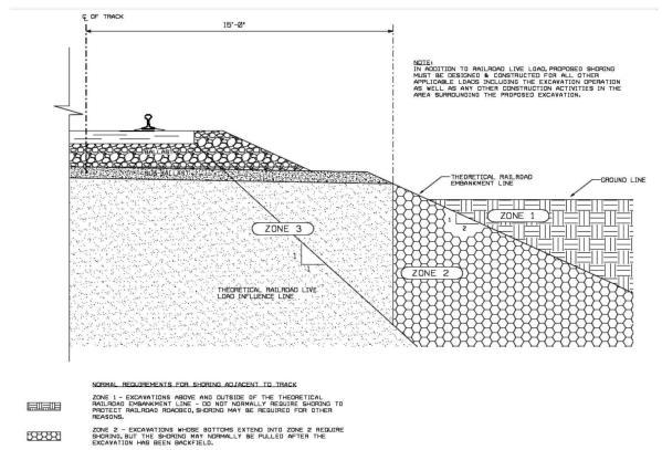
ZONE 3 - EXCAVATIONS WHOSE BOTTOMS EXTEND INTO ZONE 3 WILL NORMALLY REQUIRE THE SHORING TO BE LEFT IN PLACE AND CUT-OFF 3' BELOW BASE OF RAIL SHORING MUST BE DESIGNED FOR COOPER E60 LIVE LOAD
