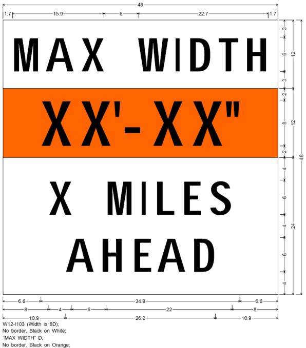
No border, Black on Orange "XX'-XX"" D; No border, Black on White; "X MILES" D; "AHEAD" D; <u>Standard 701326:</u> This standard shall apply during construction of hot-mix asphalt shoulders. This traffic control and protection standard shall be paid for at the contract unit price per lump sum for TRAFFIC CONTROL AND PROTECTION, STANDARD 701326.
