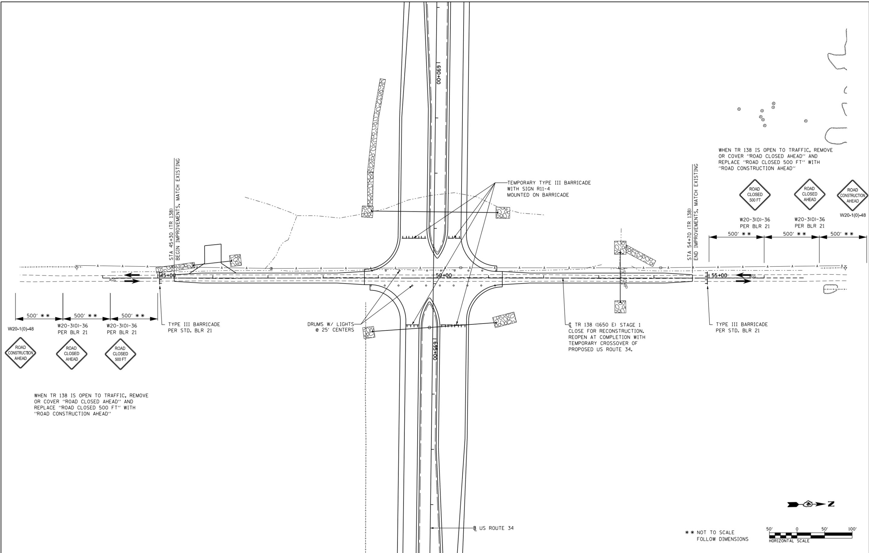
WHEN TR 138 IS OPEN TO TRAFFIC, REMOVE OR COVER "ROAD CLOSED AHEAD" AND REPLACE "ROAD CLOSED 500 FT" WITH "ROAD CONSTRUCTION AHEAD"
