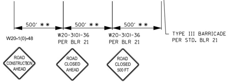
WHEN TR 138 IS OPEN TO TRAFFIC, REMOVE OR COVER "ROAD CLOSED AHEAD" AND REPLACE "ROAD CLOSED 500 FT" WITH "ROAD CONSTRUCTION AHEAD"
