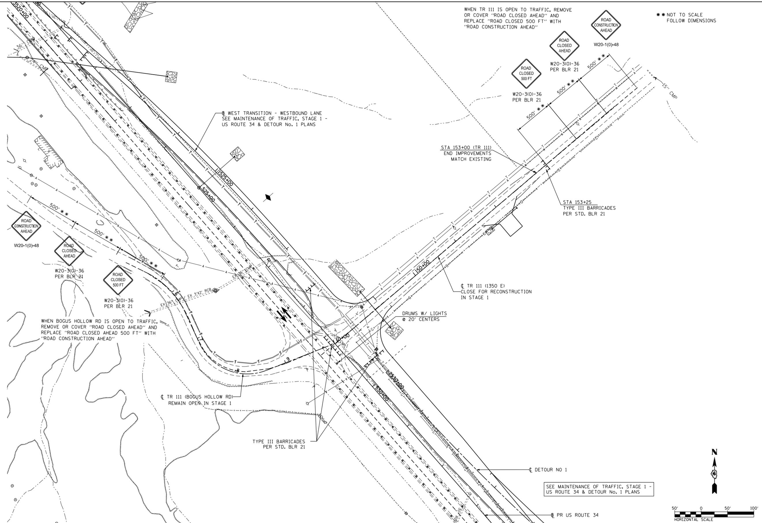
WHEN TR 111 IS OPEN TO TRAFFIC, REMOVE OR COVER "ROAD CLOSED AHEAD" AND REPLACE "ROAD CLOSED 500 FT" WITH "ROAD CONSTRUCTION AHEAD"
