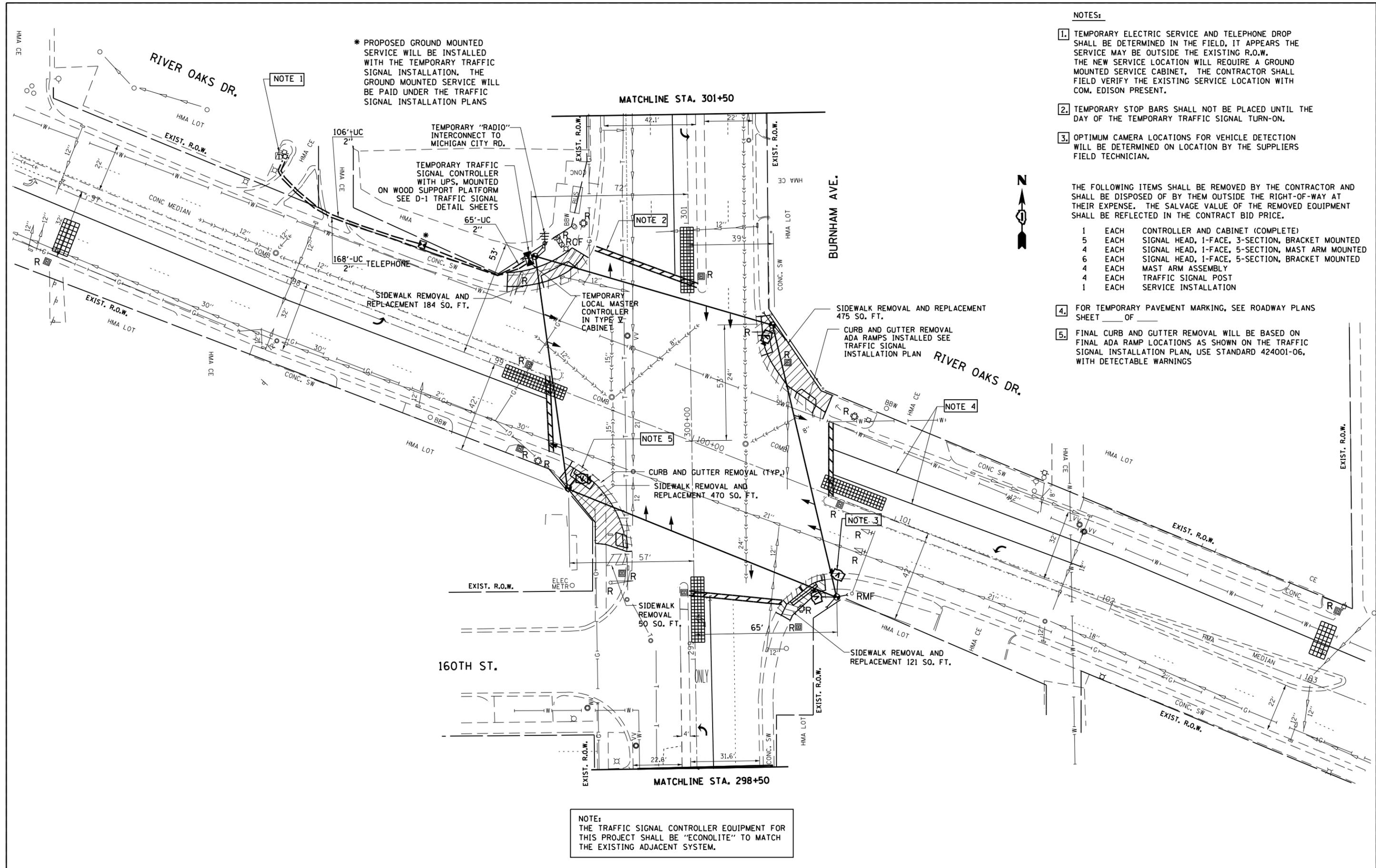
\* PROPOSED GROUND MOUNTED SERVICE WILL BE INSTALLED WITH THE TEMPORARY TRAFFIC SIGNAL INSTALLATION. THE GROUND MOUNTED SERVICE WILL BE PAID UNDER THE TRAFFIC SIGNAL INSTALLATION PLANS
