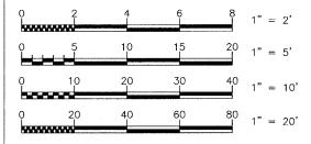
FULL SIZE PLANS HAVE BEEN PREPARED USING STANDARD ENGINEERING SCALES, REDUCED SIZED PLANS MAY NOT CONFORM TO STANDARD SCALES. IN MAKING MEASUREMENTS ON REDUCED PLANS, THE ABOVE SCALES MAY BE USED.
