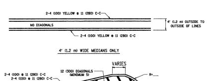
CANNOT BE ATTAINED, USE 5 (FIVE) EQUALLY SPACED DIAGONAL LINES. DIAGONAL LINE SPACING: 50' (15 m) C-C (LESS THAN 30MPH (50 km/h)) 75' (25 m) C-C 30MPH (50 km/h) TO 45MPH (70 km/h)) 150' (45 m) C-C (MORE THAN 45MPH (70 km/h))
