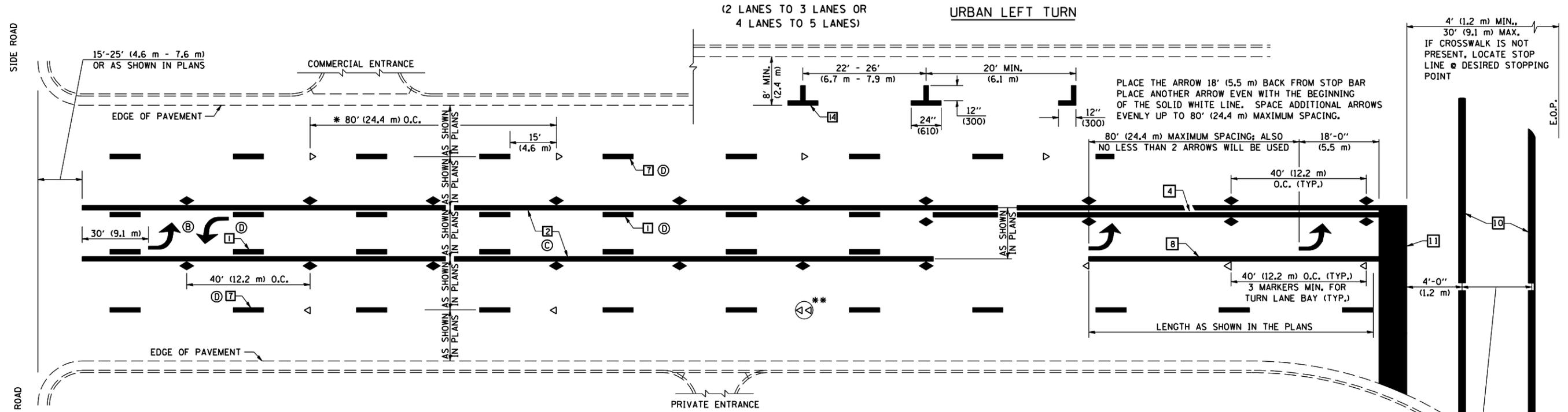
\* REDUCE TO 40 FEET (12.2 METERS) ON CENTER ON CURVES WHERE ADVISORY SPEEDS ARE 10 MPH (15 km/h) LOWER THAN POSTED SPEEDS.
