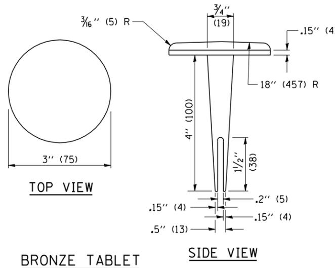
NOTE: THE CONTRACT UNIT PRICE FOR PERMANENT SURVEY MARKERS, TYPE IV, WILL BE PAYMENT IN FULL FOR FURNISHING, INSTALLING, AND PERMANENTLY MARKING ONE MONUMENT AND FURNISHING AND INSTALLING FOUR CROSS TIE MARKERS AT THE LOCATIONS SPECIFIED. THE DESIGN CHIEF OF SURVEYS MUST BE CONTACTED FOR SUPERVISION OF THE PLACEMENT AND CONSTRUCTION OF THESE ITEMS.
