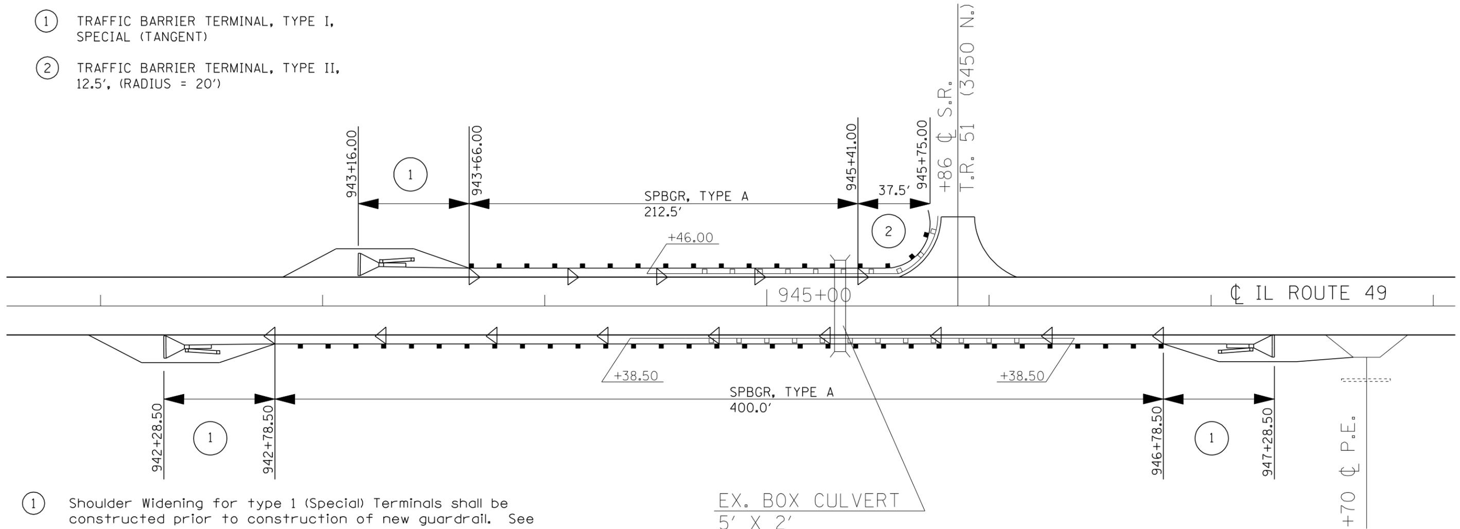
① Shoulder Widening for type 1 (Special) Terminals shall be constructed prior to construction of new guardrail. See Standard 630301-04 for Details.
