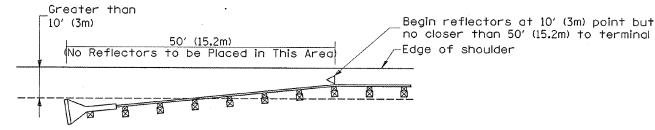
NOTE: Omit terminal marker when terminal over (10') from edge of paved shoulder or break point of unpaved shoulder.
