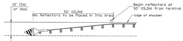
Traffic Barrier Terminal Type 1(Specia)! [Terminal 10' (3m) or less from edge of shoulder] All dimensions are in inches (millimeters) unless otherwise noted.
