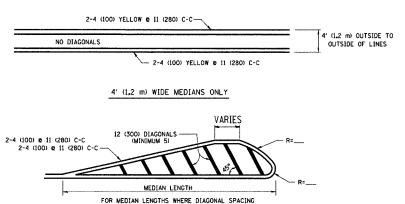
DIAGONAL LINE SPACING: 50' (15 m) C-C (LESS THAN 30MPH (50 km/h)) 75' (25 m) C-C 30MPH (50 km/h) TO 45MPH (70 km/h)) 150' (45 m) C-C (MORE THAN 45MPH (70 km/h))
