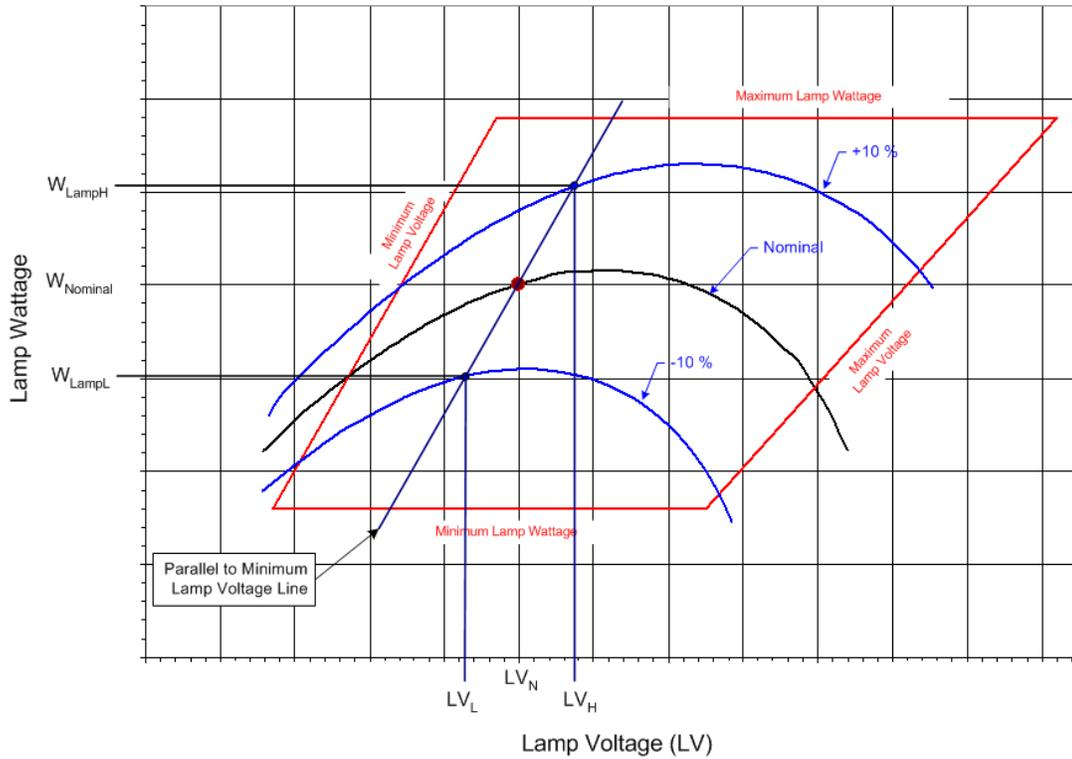
$$\text{Ballast Regulation} = \frac{W_{LampH} - W_{LampL}}{W_{LampN}} \times 100$$
