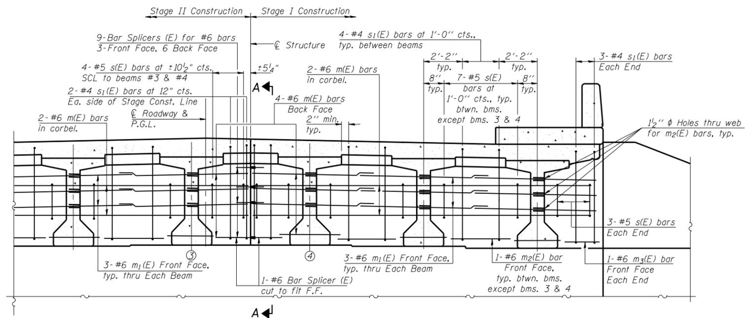
**DIAPHRAGM ELEVATION AT ABUTMENT**
